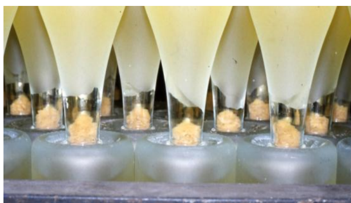
Castellblanch Cava, Penedes. Bottles neck-down in freezing solution after remuage and before automated disgorging to get rid of the yeast.
