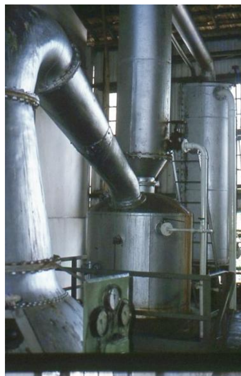
Double distillation in coconut arrack production in Sri Lanka.
