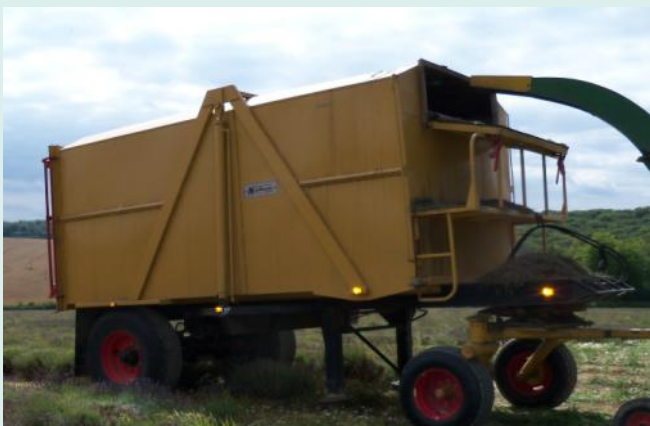
The mint being harvested with a forage harvester and being blown into a trailer/cooker tub
