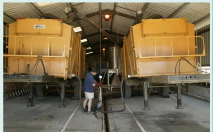
The two trailer/cooker tubs are sealed then connected to the stills ready for steam to be pumped through the mint
